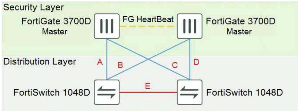
The exhibit shows a full-mesh topology between FortiGate and FortiSwitch devices. To deploy this configuration, two requirements must be met:
